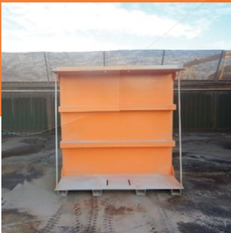
SPECIMEN NO. 1 (8.175 m²) low complex open sections
