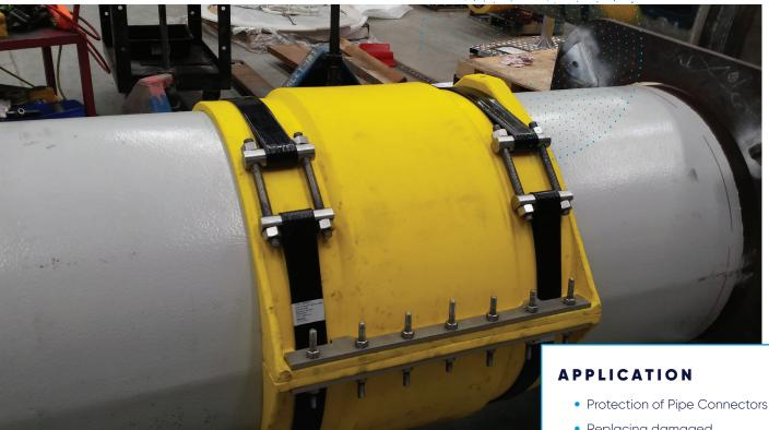
Matrix Marine Shield is a wraparound corrosion protection system for the preservation of pipelines, risers, piles and other critical field infrastructure. It may be installed at the start of service, or as a retrofit following repairs/ damage of the existing pipe/coating. Marine shield effectively seals off the encapsulated pipe from the corrosive environment, preserving its condition and extending its life.
