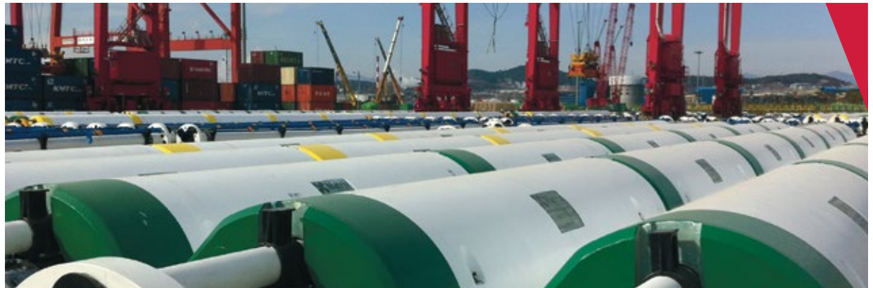
ABOVE: Riser buoyancy modules ready for deployment in Ulsan, South Korea
