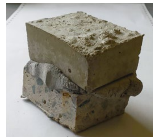
Concrete pavers bonded underwater with Paragon Aqua Grade
