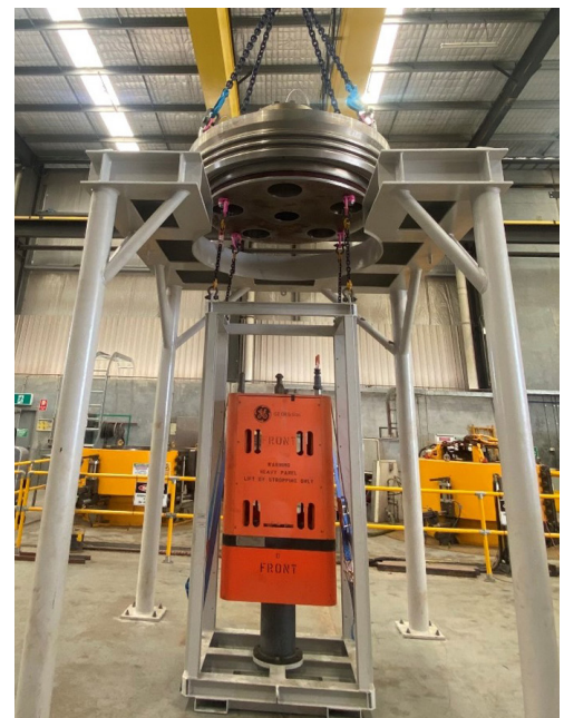
SCM ASSEMBLED INSIDE EUT FRAME HOOKED TO L1 CHAMBER LID AND SUPPORTED BY 40 T CRANE
