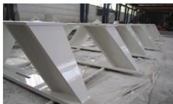
Steel supporting parts in subway stations
