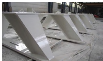
Steel supporting parts in subway stations
