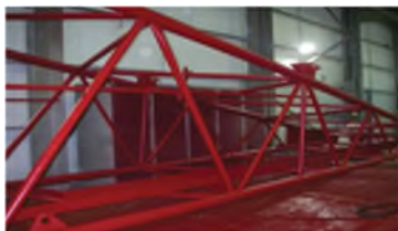
Offshore crane structure
